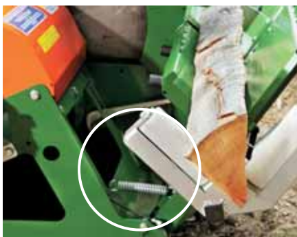
CutMaster 700 Compact, s amortiziranom klackalicom
